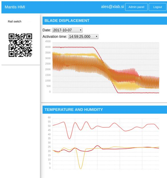
Figure 9: A dashboard for monitoring a switch
