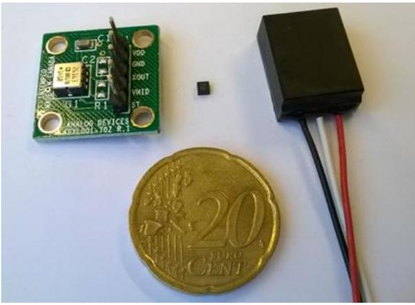
Fig. 1. Accelerometers from left: ADXL001, KX122-1037 and ACH01.
