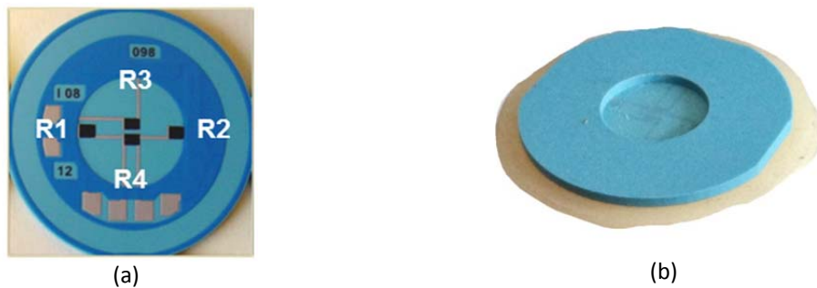
Fig. 3. (a) The front of the test structure (the diameter of the 100- \mu m diaphragm is 9.6 mm, the outer diameter of the structure is 25 mm and its thickness is 1.1 mm); (b) The back side of the test structure.
